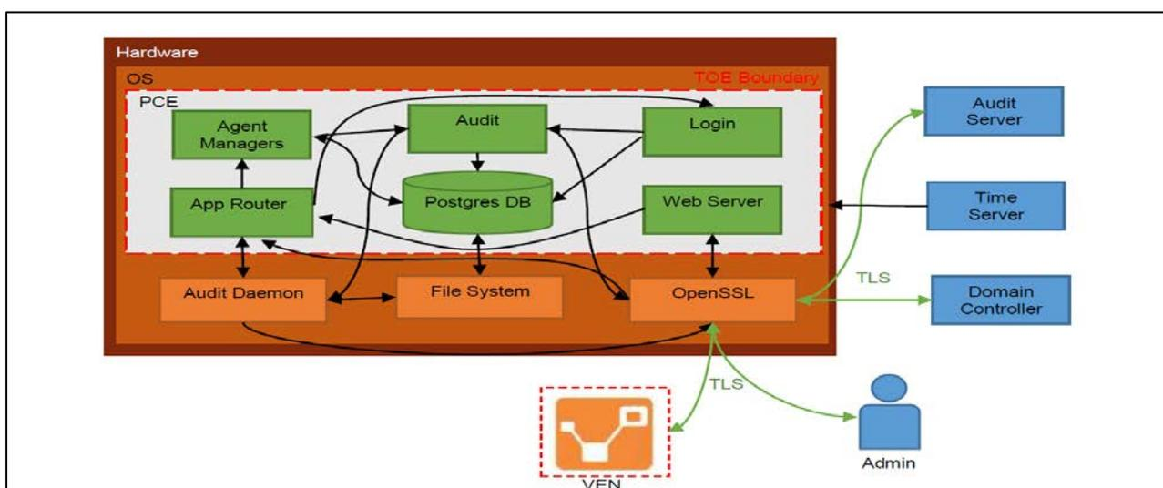
**Figure 1: TOE Architecture**
